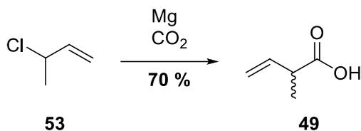
**Scheme 34.** Grignard reaction of halide **53** in preparation of 2-methylbut-3-enoic acid
