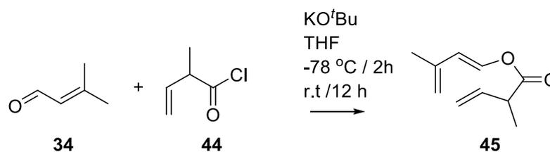
**Scheme 27.** Successful preparation of a different linear triene **45**. Yield not determined
